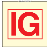
59. Inert gas installation
