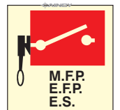
36. Remote controlled fire pumps or emergency switches
