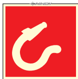
32. Hose box with spray/jet fire nozzle
