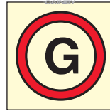
152. Emergency source of electrical power (generator)
