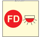
6. Space protected by automatic fire alarm
